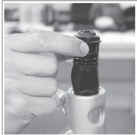
Figure 44 Removing the SPV Damping Assembly
