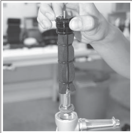
Figure 45 Removing the SPV Damping Assembly
