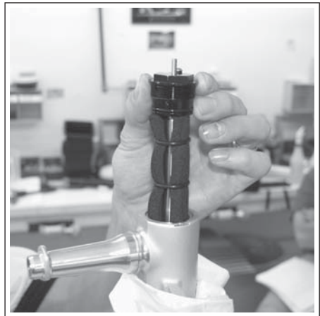
Figure 50 Inserting the TPC Damper
