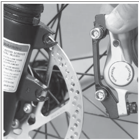
Figure 12 Lefty Brake Caliper Off
