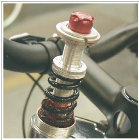
Figure 26 Outer Cap Assembly Removal
