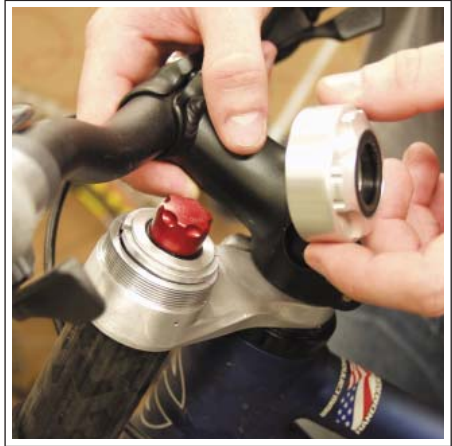
Figure 24 Outer Cap Assembly Removal
