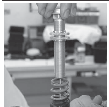
Figure 34 Lifting Off the Shaft
