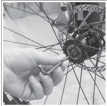
Figure 15 Lefty Loosen Brake Caliper
