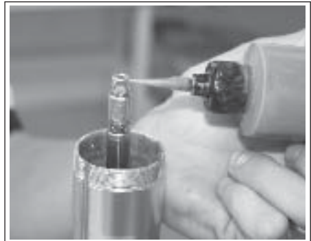
Figure 36 Apply Loctite #242 (blue) to the threads.
