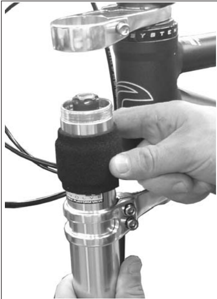
Figure E Lefty Alloy Fork Removal
