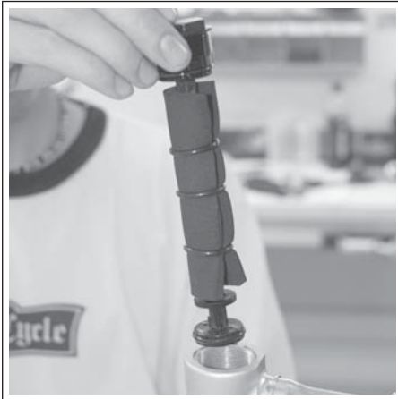
Figure 46 Removing the FFD Damping Assembly
