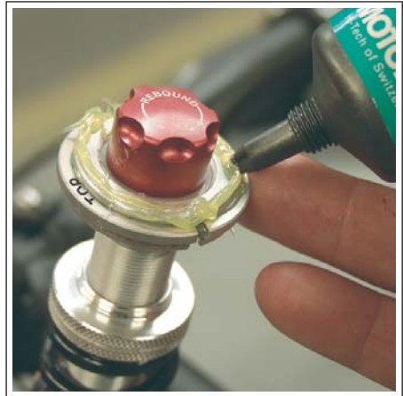
Figure 30 Tighten Lock Ring Securely
