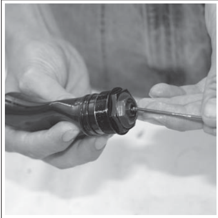
Figure 49 Expanding the SPV Bladder
