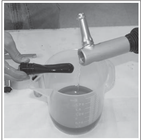
Figure 47 Draining Oil From The Lefty
