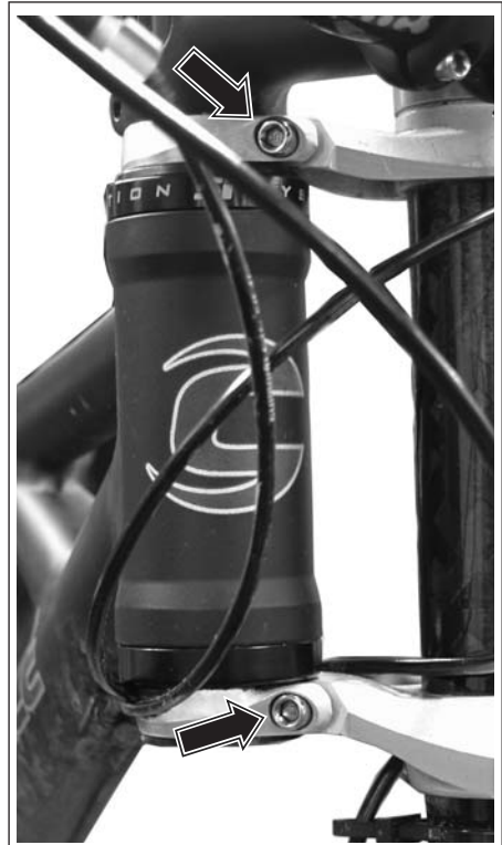
Figure D Lefty Carbon Fork Clamp Bolts
