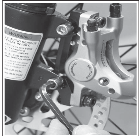
Figure 11 Lefty Loosen Brake Caliper
